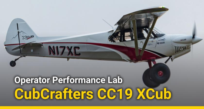
**Short Takeoff And Landing (Stol) Testbed For Low-Altitude Sensor Research**
